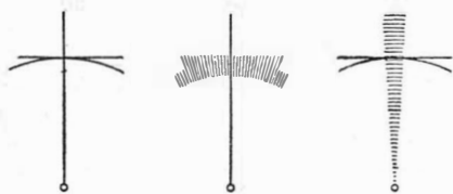
FIG. 25. ASTIGMATISM OF CONCENTRIC CIRCLES
