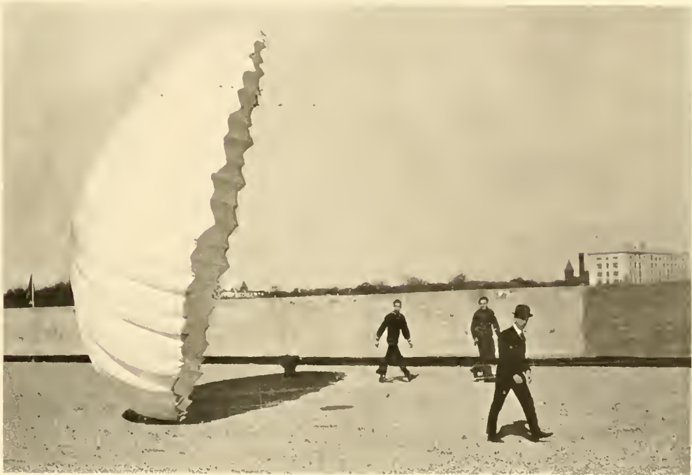
SILK PARACHUTE IN WIND Showing Shape When Open and Size Relative to Man
