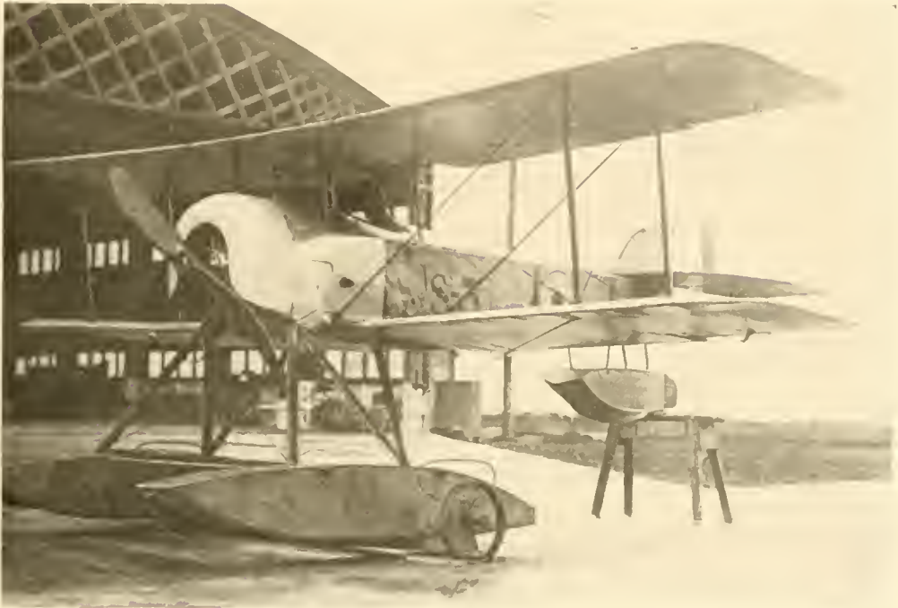
SOPWITH MACHINE CONVERTED FOR WATER WORK BY ADDING PONTOONS
